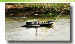
HydroBoard II: Dive resistent design for use in normal or extreme flow conditions.
