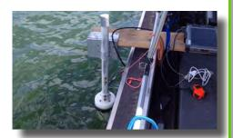
Boat Mount: Delrin/aluminum fixture designed to facilitate mounting over the side of a boat.
